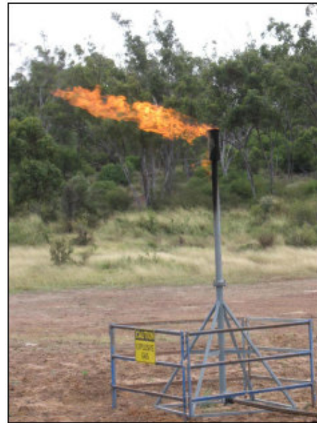
Gas Flare from recent Fort Cooper Coal Measure Pilot Well
